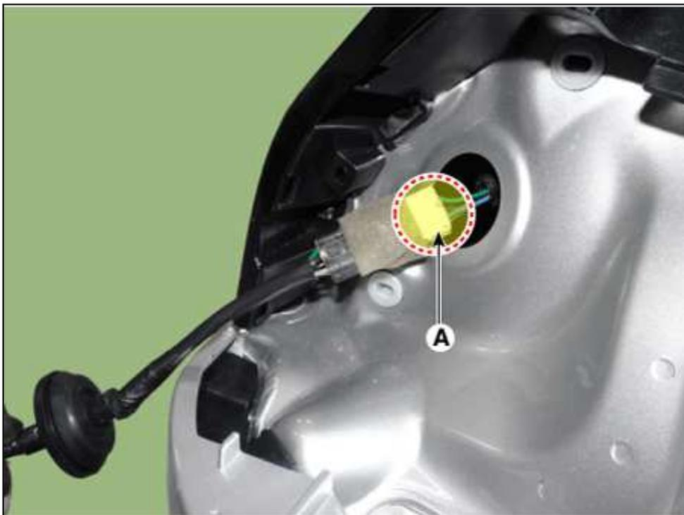
5. Loosen the rear bumper upper mounting fastener.
