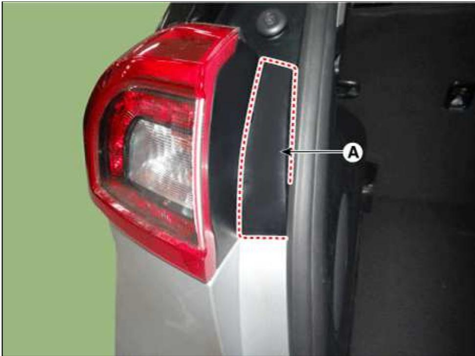
2. Remove the rear combination lamp (A) after loosening the mounting screws.
