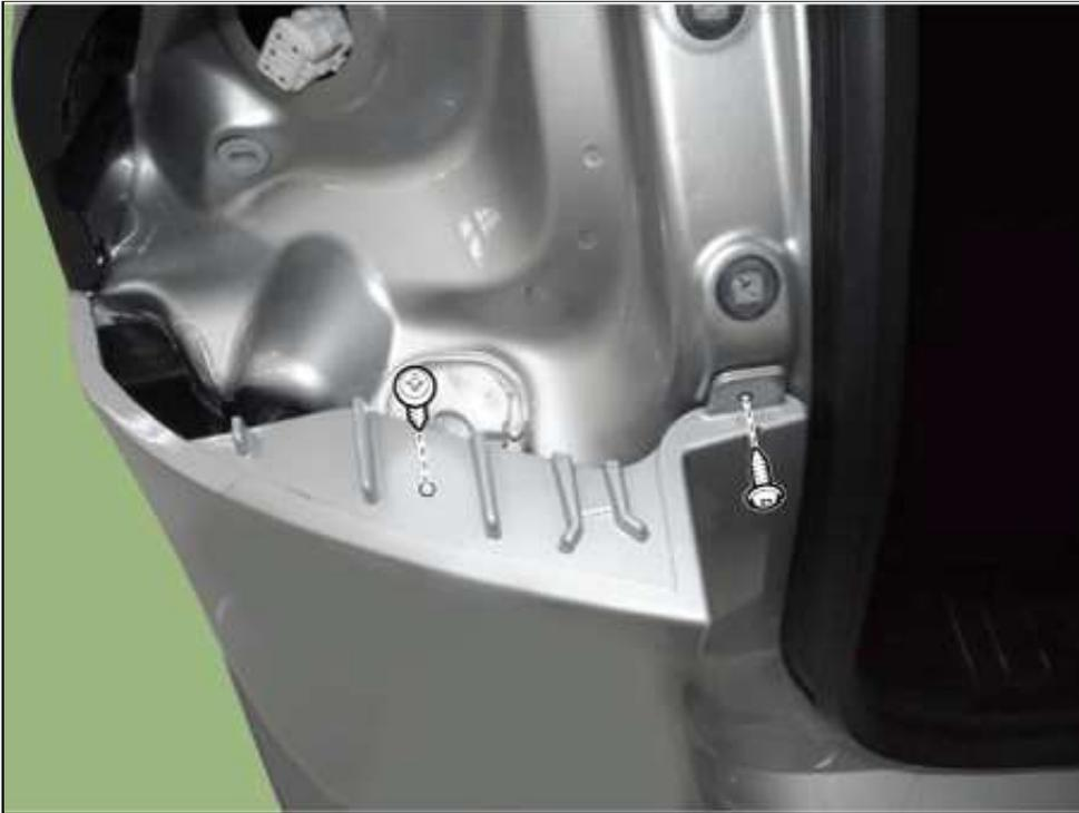
6. Remove the rear bumper side after loosening the screw and fastener.
