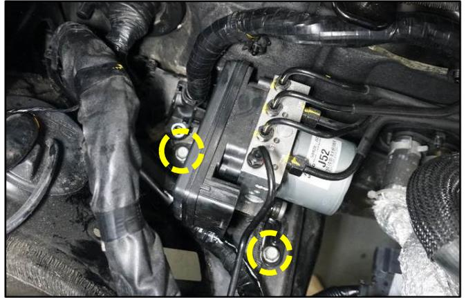
38. Detach the two (2) wiring harness retaining clips.
