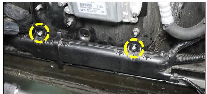
46. Detach the Multipurpose Check connector (W1) from the vehicle and disconnect the A/C Pressure Transducer connector (W2). Detach the wiring harness retaining clip.
