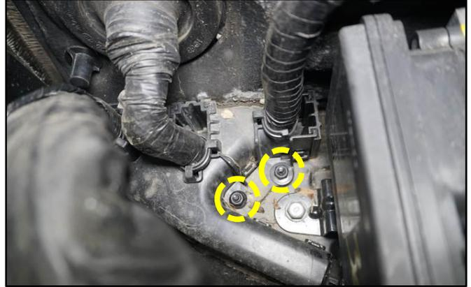
35. Remove the ground cable and grommet (V1) located next to the Electronic Stability Control (ESC) module (V2).
