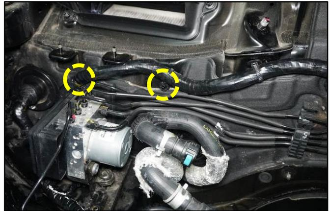
39. Detach the grommet (V4) from the firewall, located behind the ESC module (V2) and pull out connector (D2) removed in step 4 of this procedure.
