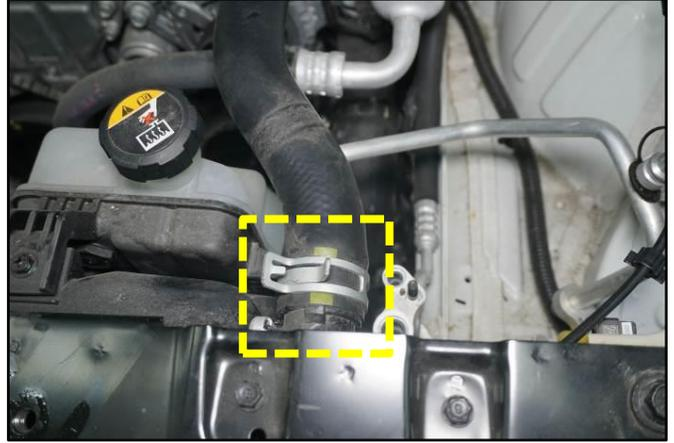
8. Detach the transmission oil cooler inlet and outlet pipes (B1) from the transmission cooler.
